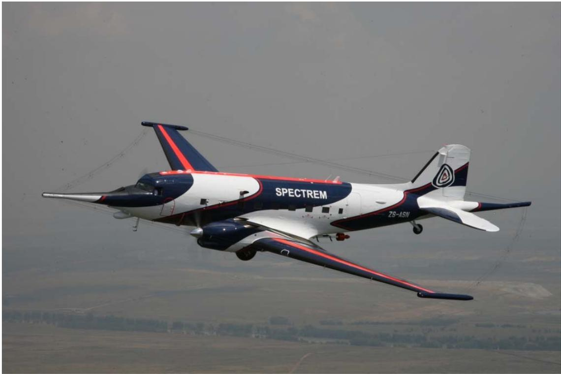
Figure 1. Anglo American's proprietary "Spectrem" EM system.
