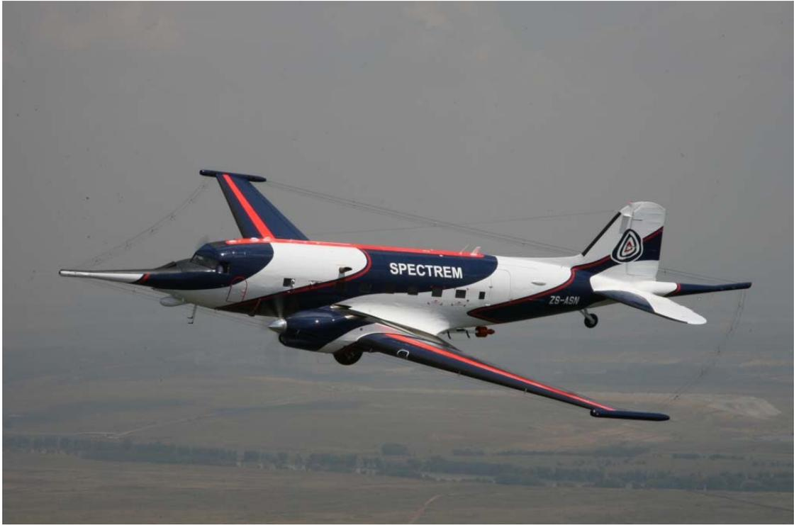
Figure 2. Anglo American's proprietary "Spectrem" EM system.
