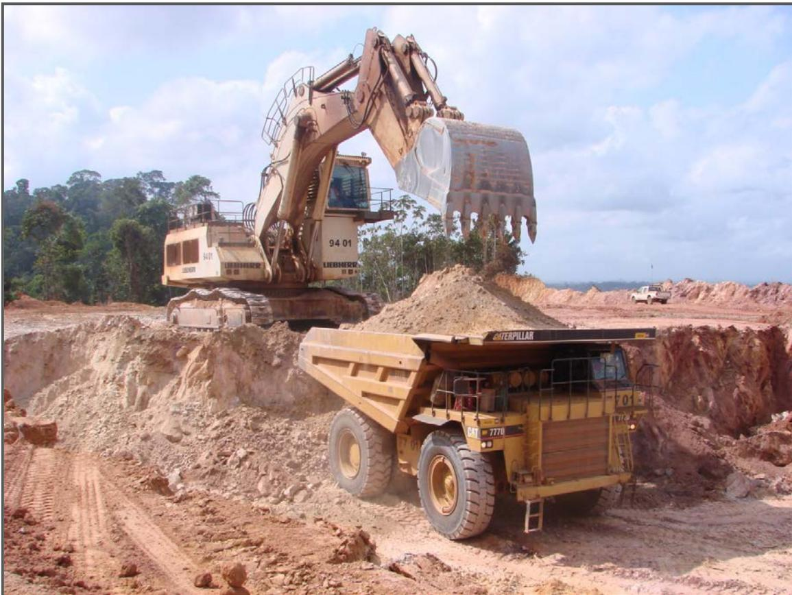
**Photo 6 – Liebherr 994 loading a Cat 777 at the Tap AB Eastern wall cutback.**
