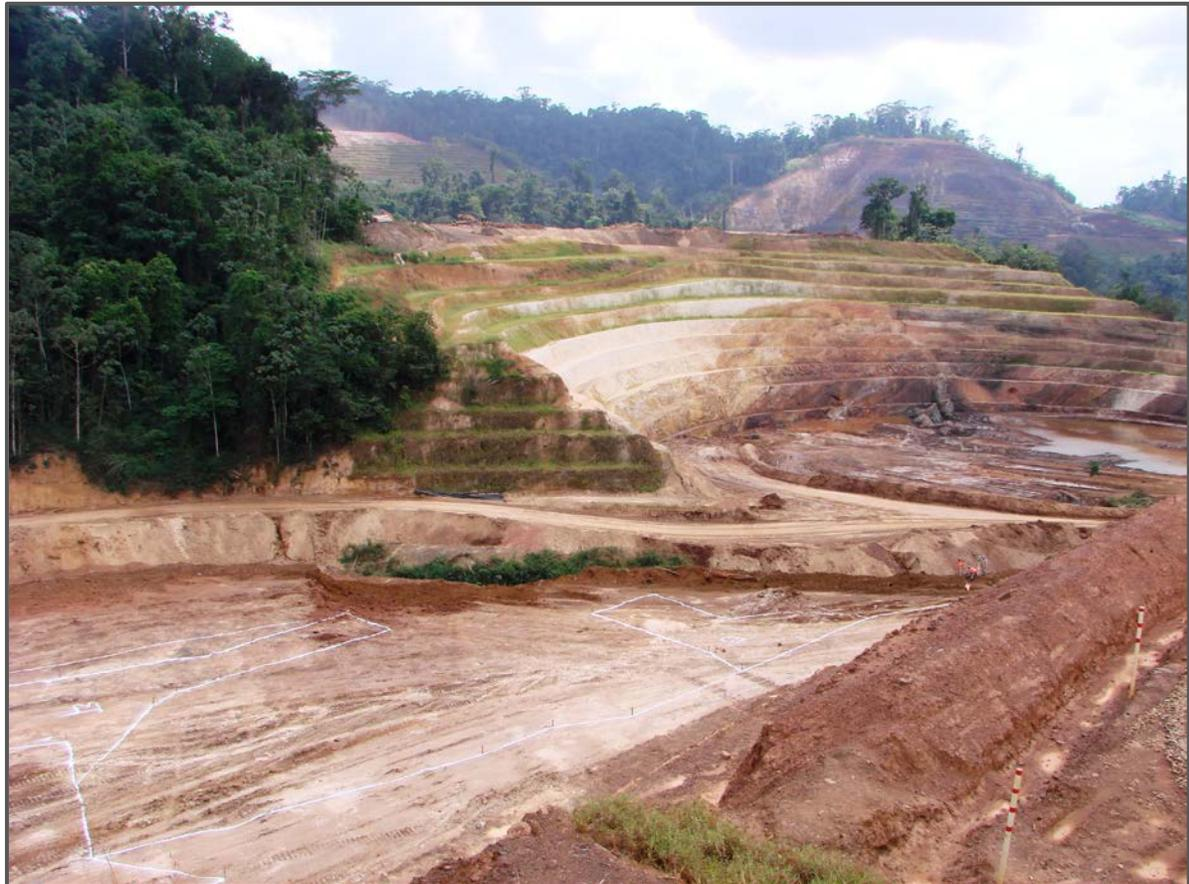
**Photo 4 – Tap D2 pit in background with ore mark-up on a Tap D3 bench in the foreground**
